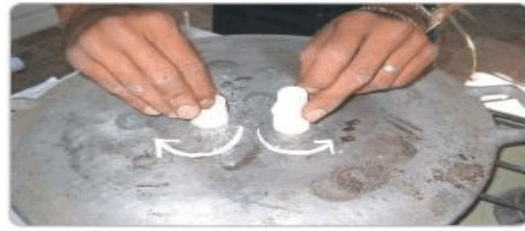
Heat the edges of the male adapter (right) and the piece cut off the female adapter (left), turning them around their axis on the hot plate, until they turn around easily in their own melt.
