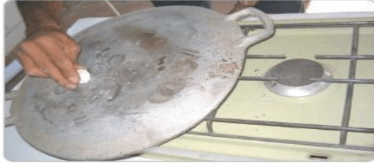
Heat the metal (aluminum) sheet. Test the temperature with a piece of PVC. The plate should not be so hot as to “burn” the PVC (turning it brown).
