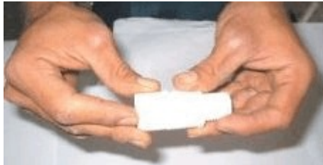
Heat the metal (aluminum) sheet. Test the temperature with a piece of PVC. The plate should not be so hot as to “burn” the PVC (turning it brown).
